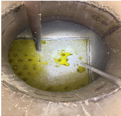
图9 发生凝固时的熔盐状态 Fig. 9 Molten salt condition during solidification
