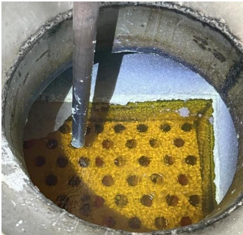
图8 加热至580℃且恒温48小时后的熔盐状态 Fig. 8 State of the molten salt after heating to 580℃ and holding at that temperature for 48 hours
