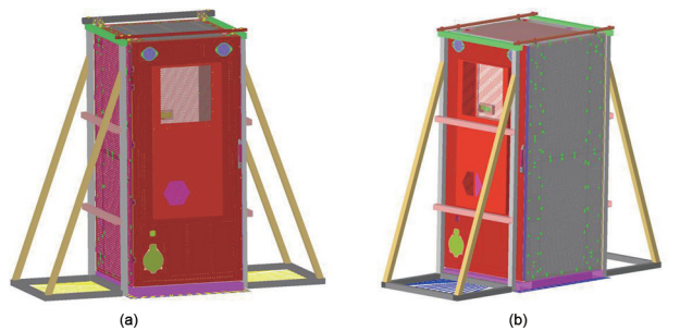
图9 z向随机振动现场图 Fig. 9 Laboratory setup for random vibration test on z-axis
