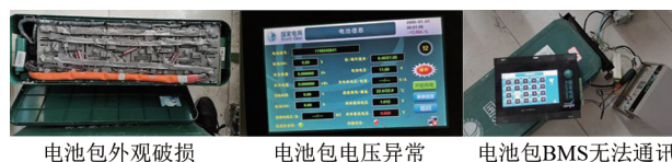
图2 电池包初选结果 Fig.2 Results of initial filtration
